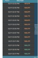
When in the Patch Detail screen monitoring an individual patch, select the "History" button to view a list of temperature measurements for a more detailed look at the temperature changes over time. You may also tap the icon in the upper right of this screen to export data via e-mail. The data is sent as a .csv file which can be viewed in Microsoft® Excel®.
